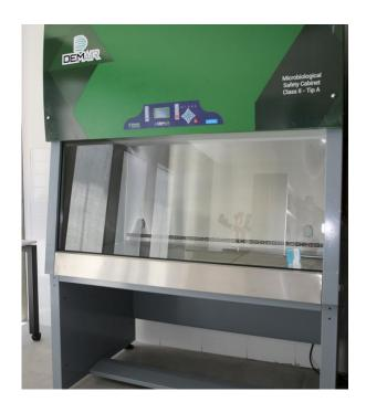
**Intended Use of the Instrument:** It is designed specifically to protect working personnel and the environment from infectious aerosols and splashes. It provides a sterile environment for the experiment.
